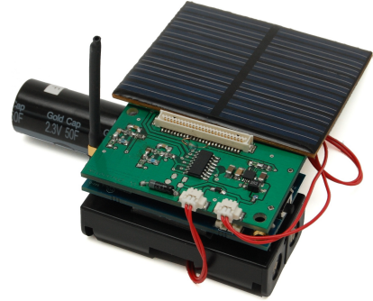
Figure 9: Energy harvesting power supply for the IRIS platform with a solar cell and supercapacitor energy buffer
