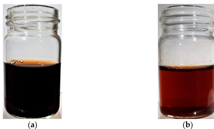
Figure 7. Hydrolysates obtained after 70 min of hydrothermal treatment of raw digestate (a) and washed digestate (b).
