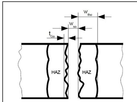
Fig. 1. Heat affected zone (HAZ) at cutting edge
