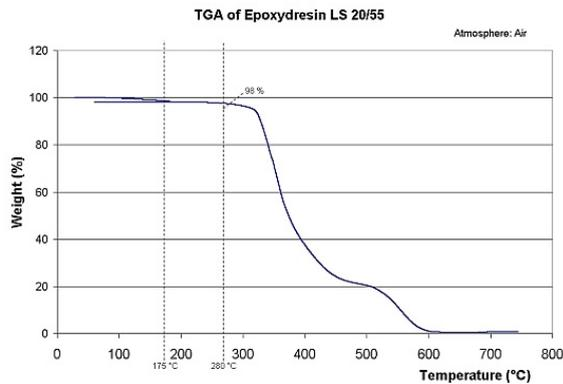
Fig. 2. Thermogravimetric analysis of a epoxy resin
