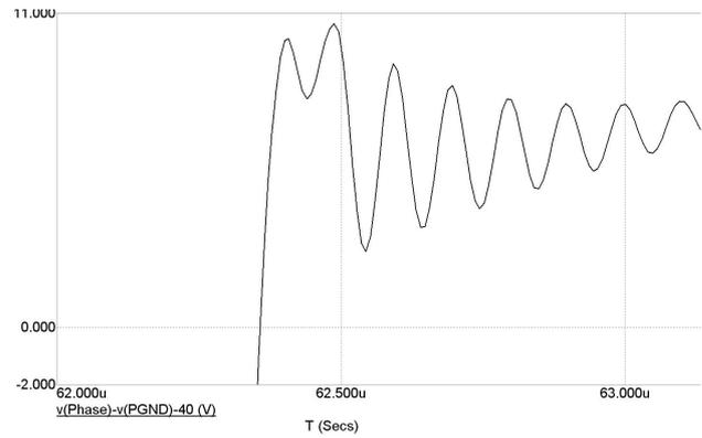
Fig. 3. Waveform of the phase voltage at a comparatively short dead time where a cross current occurs.
