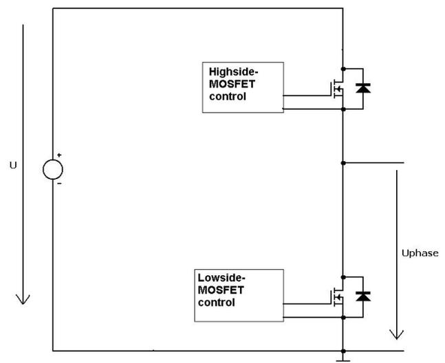
Fig. 1. Principal circuit diagram of a half bridge.
