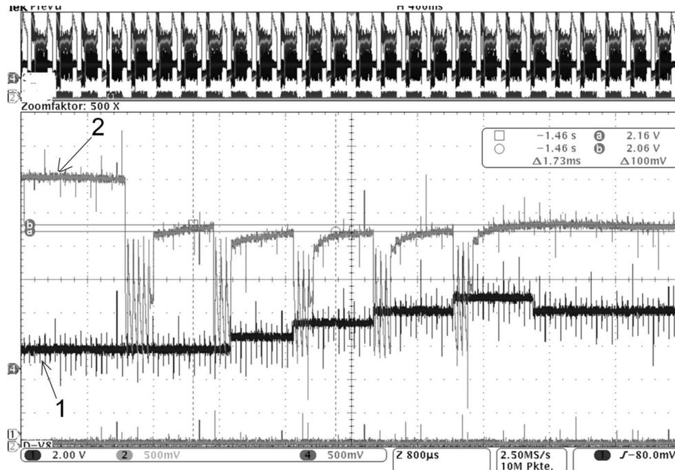
**Fig. 7.** Dead time optimization process. Curve 1: output of the DA-converter, proportional to dead time: an increase of the DA output voltage corresponds to a decrease of the dead time. Curve 2: measured voltage over the peak detection capacitor C3.
