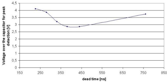
Fig. 5. Voltage across the capacitor for peak detection.
