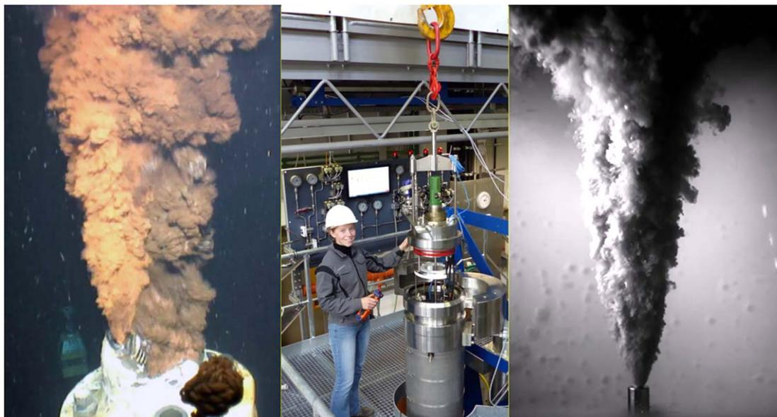
**Figure 1.** Left, escaping oil, gas and water from the top of the severed blowout preventer of *Deepwater Horizon*. Center, high-pressure oil spill simulation module, Hamburg University of Technology (TUHH). Right, simulated high-pressure oil blowout of methane-saturated oil imaged in the TUHH facility. The pipe diameter of DWH was ~0.5 m diameter (left), the TUHH experiments used a 1.5 mm orifice (right).
