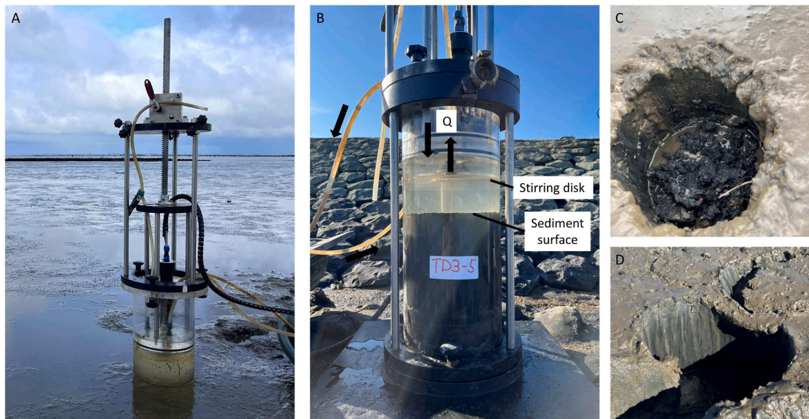
Fig. 3. A) In-situ erosion experiment in a tidal mudflat with the C-GEMS. B) Ex-situ (field) experiment with an extracted sediment core directly at the sampling site. Measuring chamber, controllers and battery pack are stored on a mud sledge outside pictures A and B. C-D) Surface of the mudflat during TD1 (C) and TD2 (D). The hole in each of the latter pictures has a diameter of 20 cm.
