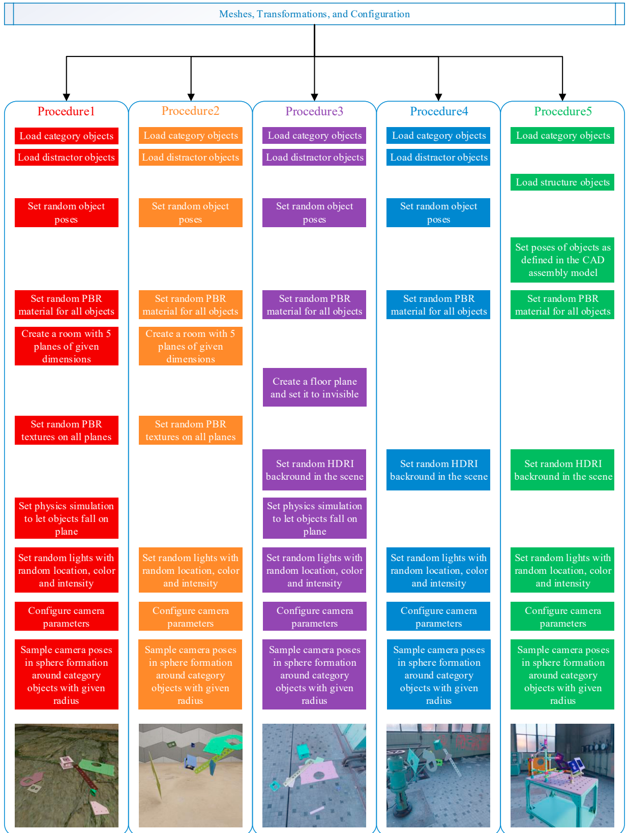
Fig. 4. Five basic data generation procedures explained in top-down approach
