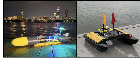
Fig. 4: Platforms used for field experiments: (left) an MIT Spurdog AUV, (right) a Clearpath Heron ASV.
