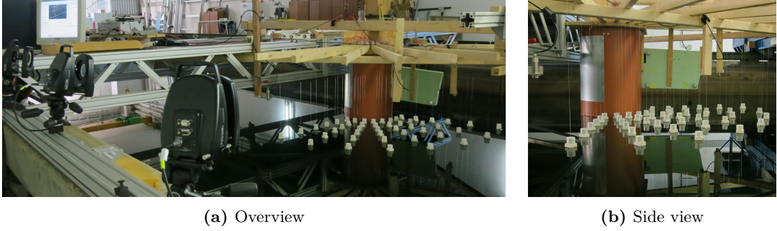
Figure 4.5.: Test setup for measurements of the diffraction caused by a cylinder
