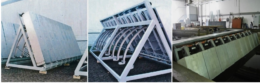
Figure 4.2.: Wave maker of the towing tank of Hamburg University of Technology (TUHH)
