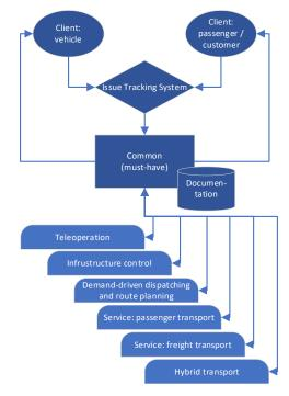
Figure 1: Conceptual modular design of an operations control center (OCC)
