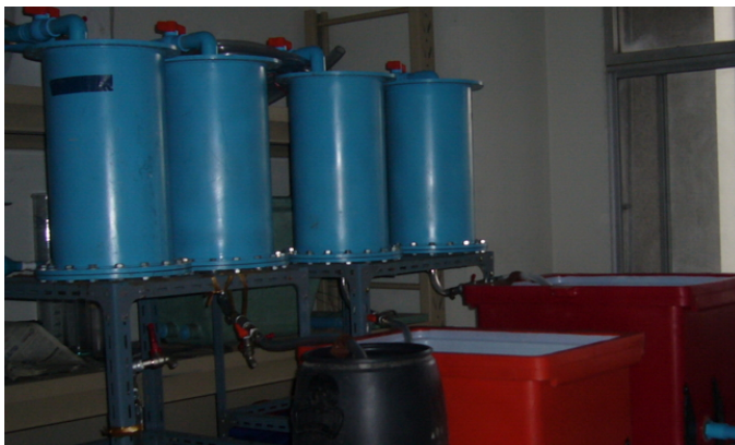
Figure 4.7: Photo showing the lab-scale swine wastewater treatment configuration in Thailand
