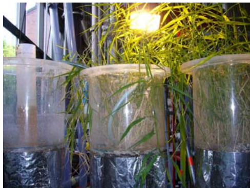
Figure 4.3: Photo showing the pilot-scale VSFCWs experiments in Germany
