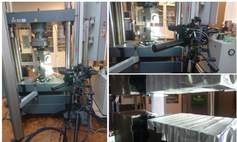
Fig. 6 Photographs of experimental setup for tensile testing with additional Digital Image Correlation system (DIC) with overall setup (left), detailed photograph of camera location (top right) and detailed photograph of a sample in the test setup (bottom right)
