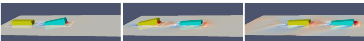
Fig. 3: Snapshots of overset-grid simulation for a generic towing operation
