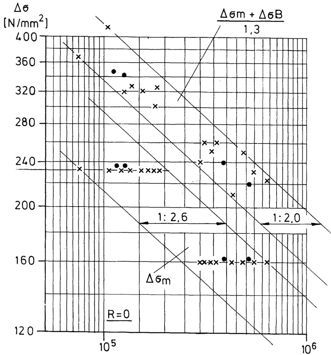
Fig. 12 Comparison of scatter bands for data from zero-to-tension load test
