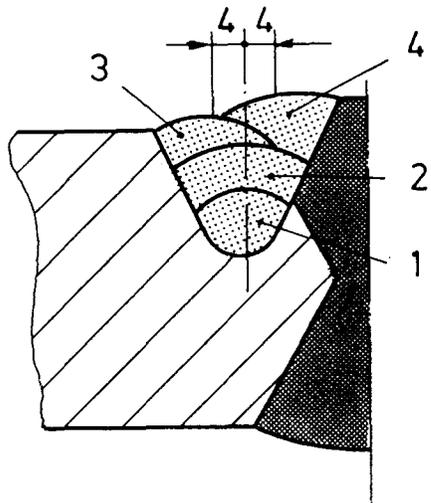
Fig. 3 Welding sequence repair weld
