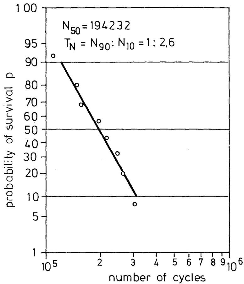
Fig. 8 Evaluation of constant amplitude load test (series 12 )
