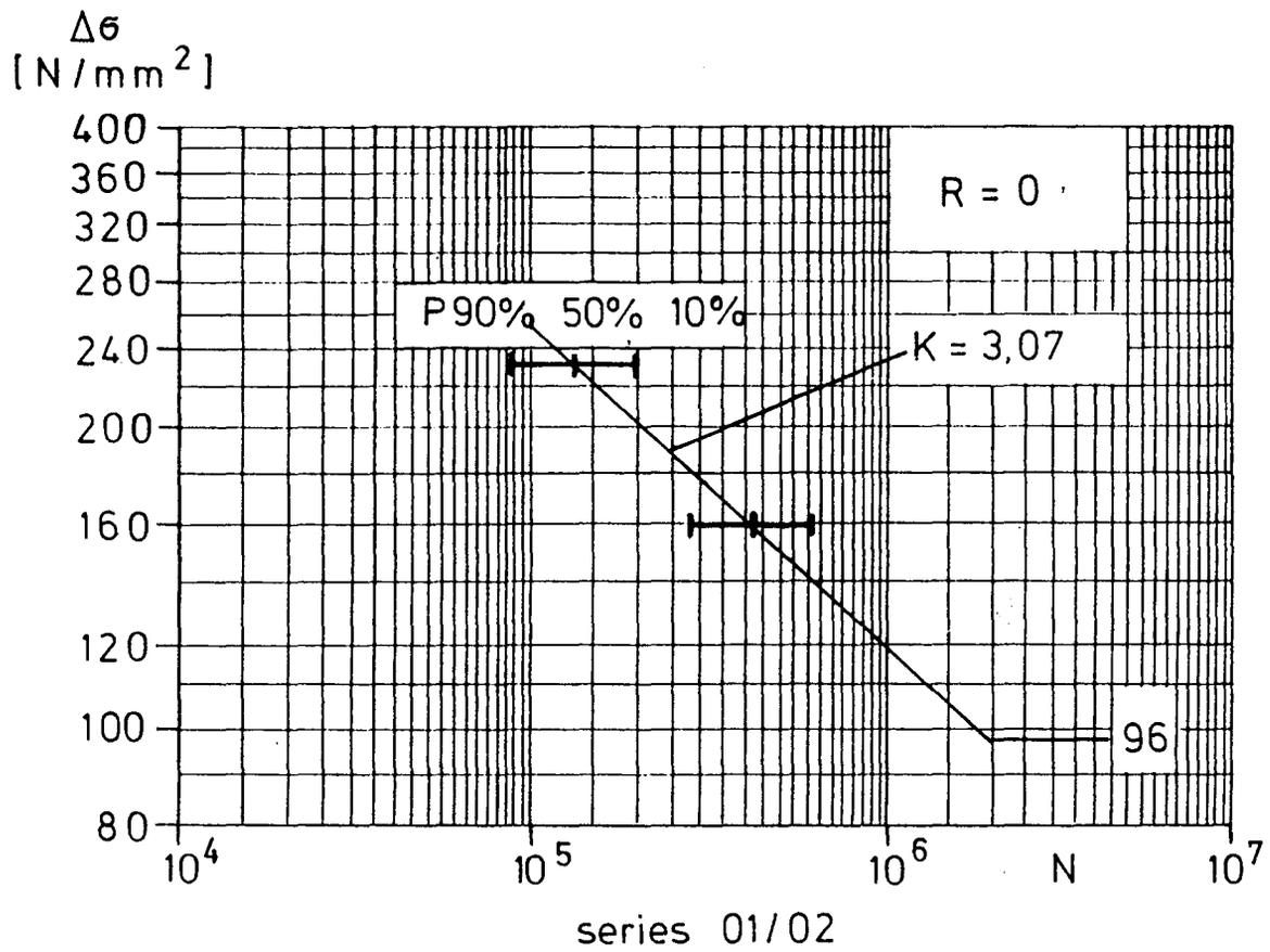
Fig. 9 S-N curve for zero-to-tension load
