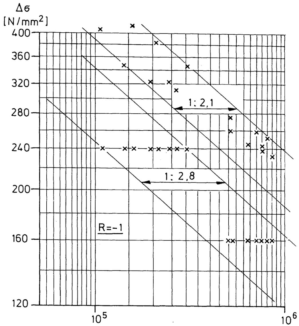
Fig. 13 Comparison of scatter bands for data from alternating load test
