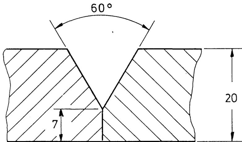
Fig. 1 Edge preparation for SAW butt weld
