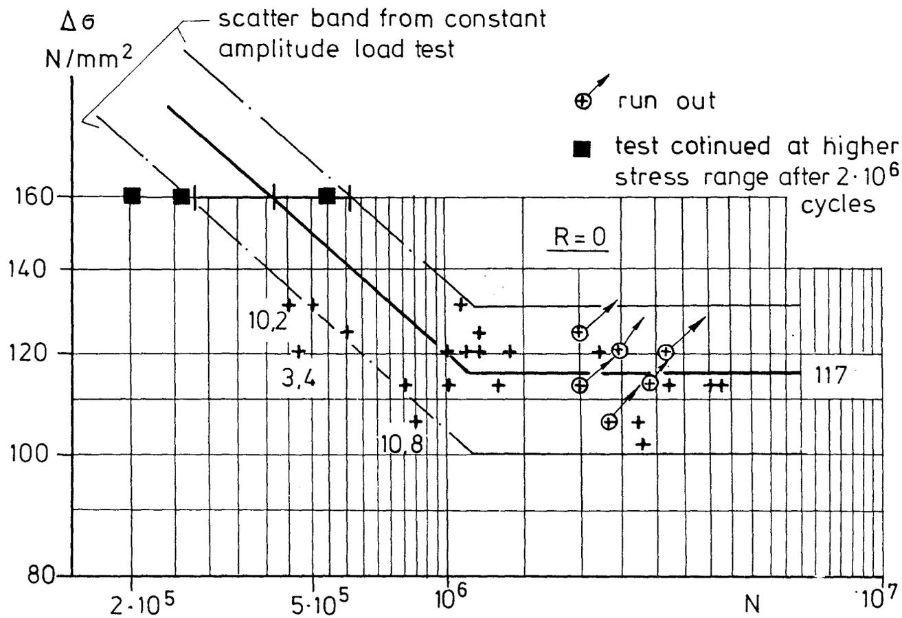
Fig. 15 Staircase test - individual test data
