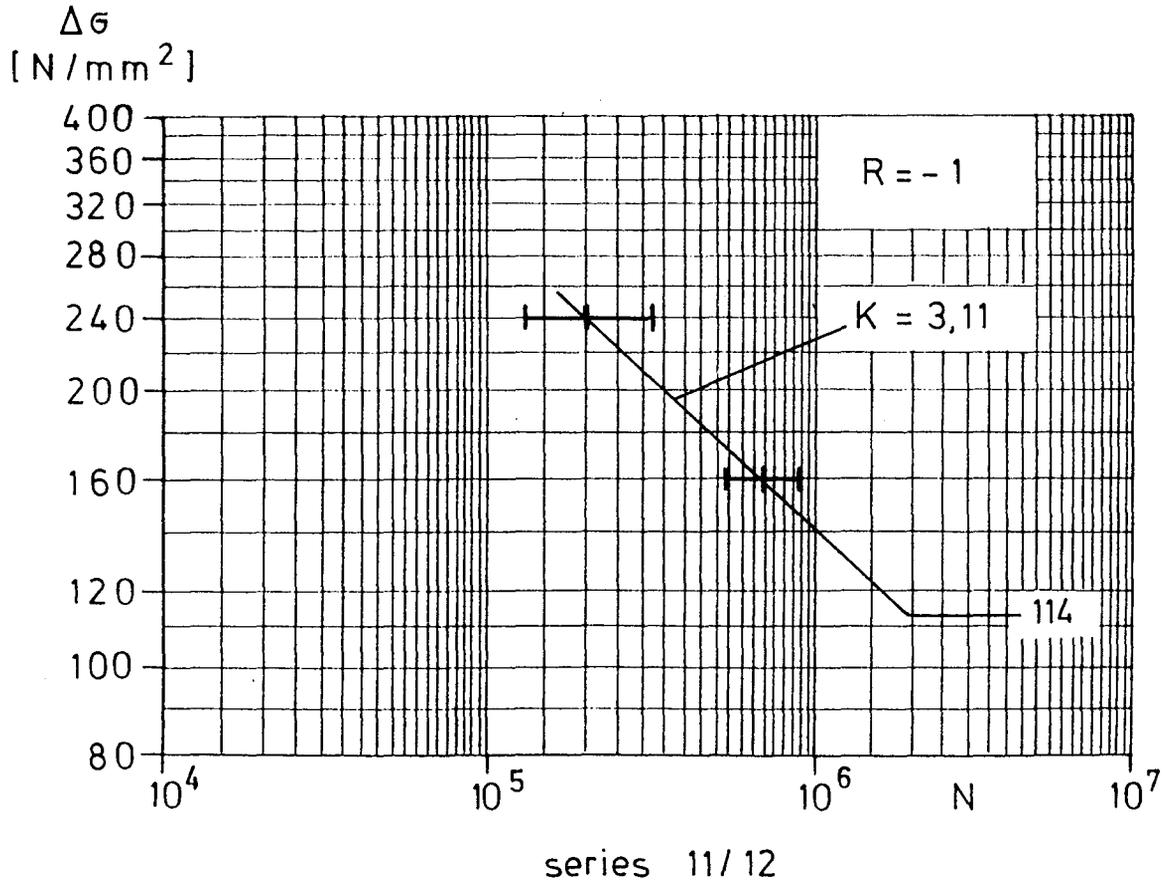
Fig. 10 S-N curve for alternating load
