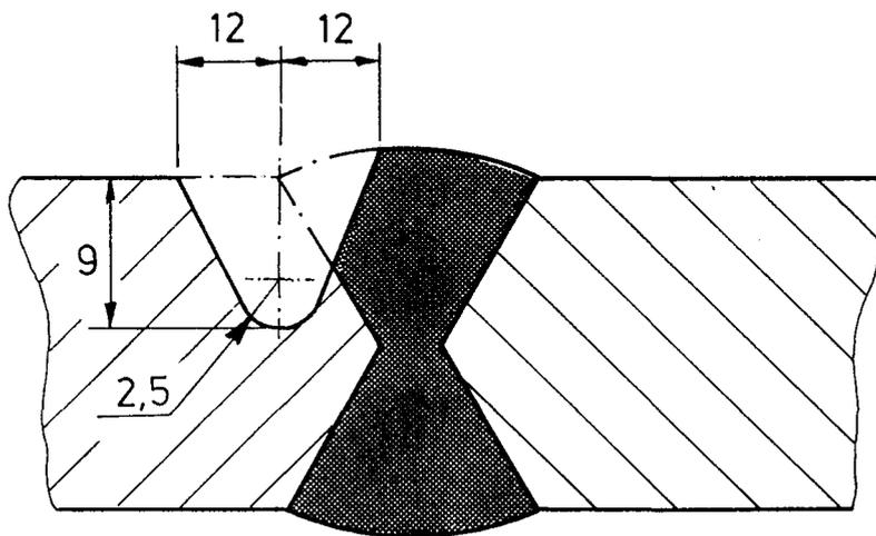
Fig. 2 Edge preparation for repair weld
