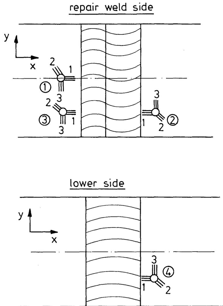
Fig. 7 Arrangement of strain gauges for residual stress measurements
