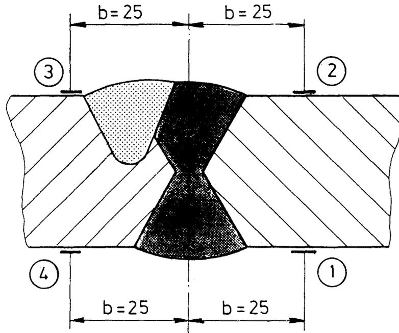
Fig. 5 Arrangement of strain gauges for secondary bending stress measurements
