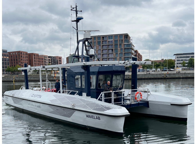
Fig. 1: The research vessel MS Wavelab in the Kiel Fjord: For remote and autonomous operation, the ferry features 5G and Starlink connections, cameras, LiDAR, and mmWave sensors.
