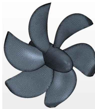
Figure 7 The close-up view shows the meshing arrangement around the tip-rake propeller.
