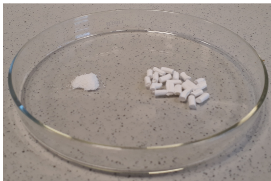
Figure 4.1: TS-1/SiO 2 pellets and TS-1/SiO 2 splits
