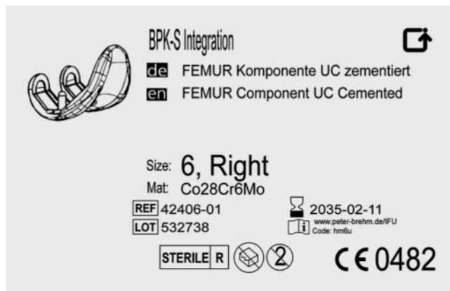
► Fig. 1 Current label for a knee implant (femoral component), showing the use of standardised symbols in accordance with DIN EN ISO 15223-1:2019. Reproduced with permission from DIN – Deutsches Institut für Normung e.V., Berlin.
