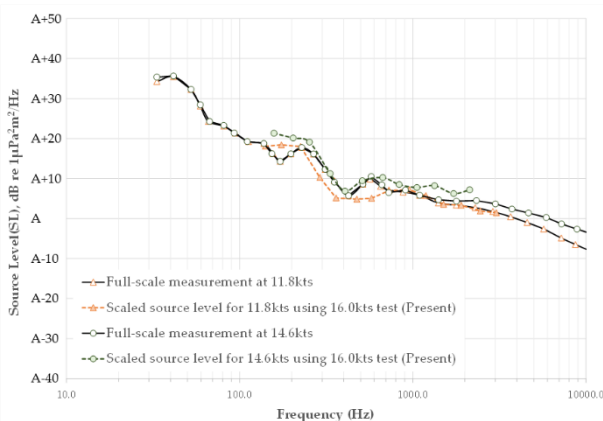
Figure 23. Comparison between the full-scale measurement results at 11.8kts and 14.6kts by Lee et al. (2012) and the scaled source level using the model test result at \sigma_{n,m} same as the full-scale cavitation number at 16.0kts
