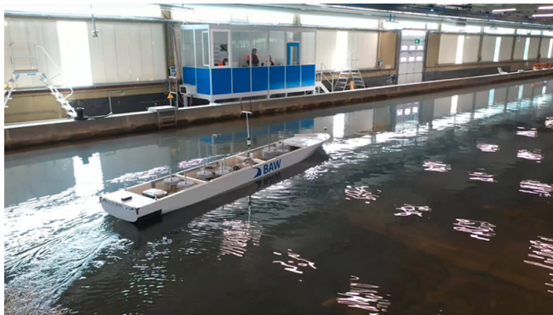
Fig. 3. DTC model ship during manoeuvre in the BAW shallow water basin.
