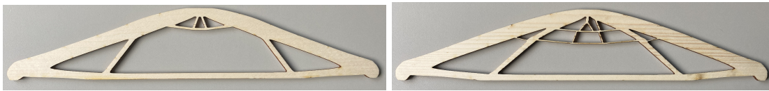
Figure 5.11: Image of the fabricated specimen. Left: deterministically optimized design, Right: robust optimized design.
