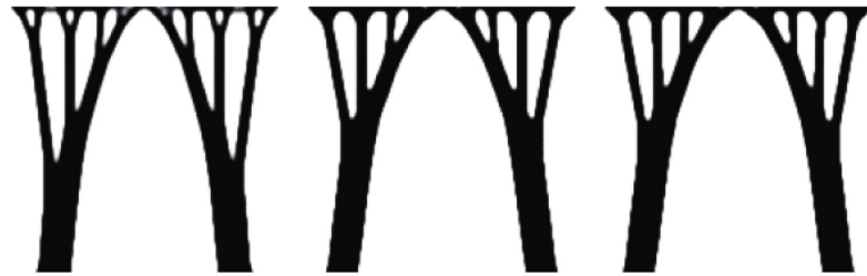
(a) Deterministic optimized design. (b) Robust optimized design using aPSF/adjoint method. (c) Robust optimized design using nPSF.
