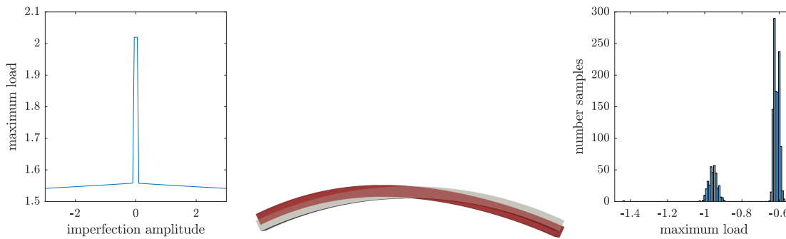
Figure 4.3: Design response of a deterministically optimized shallow arch with respect to the amplitude of a predefined imperfection (left) and a visualization of the corresponding imperfection (middle). The grey structure represents a simple perfect geometry, the red structure represents the corresponding imperfect geometry at an imperfection amplitude of 10. The right figure shows the histogram of a Monte Carlo simulation considering multiple imperfection modes.
