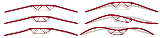
Fig. 9 EOLE modes of the 2D shallow arch example. Grey: perfect structure, red: structure with perturbation into corresponding mode direction. (Color figure online)
