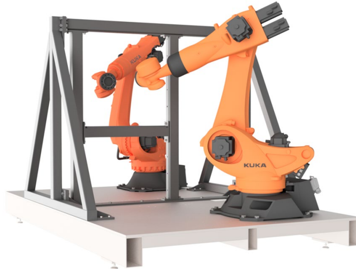
Figure 2 – Base platform consisting of machine bed, robots and frame
