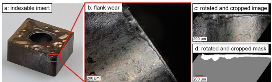
Fig. 2 Example of flank wear and image pre-processing
