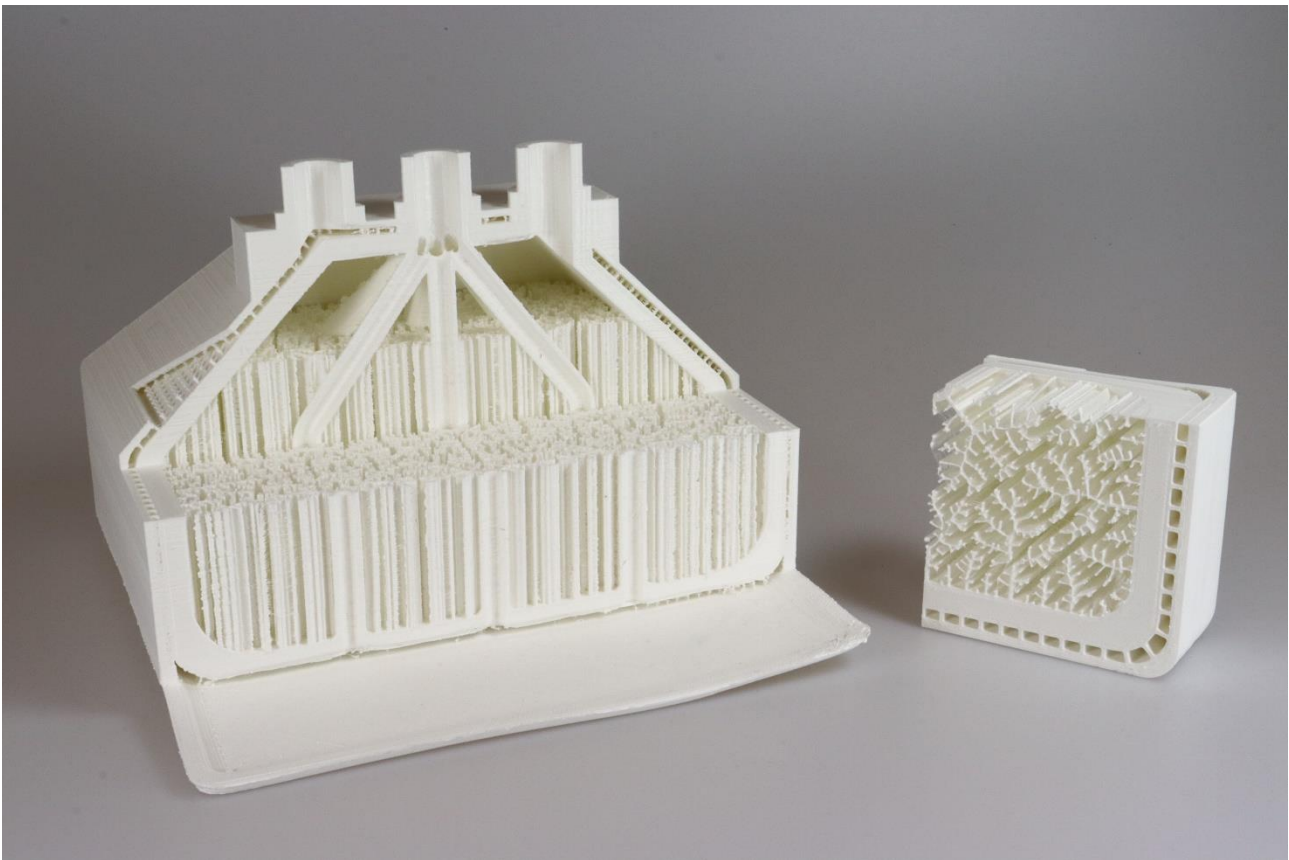
Figure 6: PLA demonstrator of the designed metal hydride tank showing the interior of the tank and an excerpt of the heat exchange structure.
