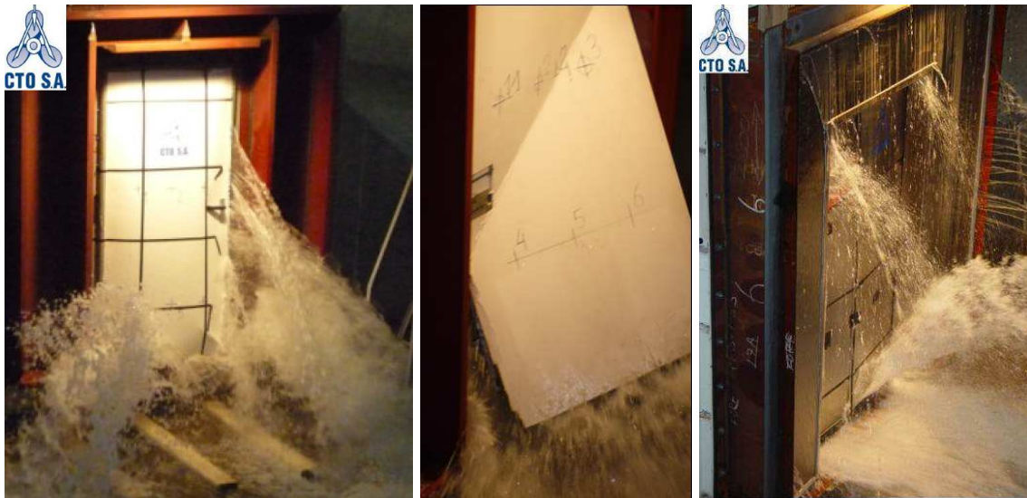
Figure 3.7: Photos of the leakage and structural failure of semi-watertight doors during model tests (Ruponen and Routi, 2011)
