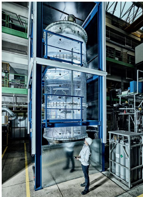
**Figure 1.** Photo of the acrylic glass reactor at the Institute of Multiphase Flows [18].
