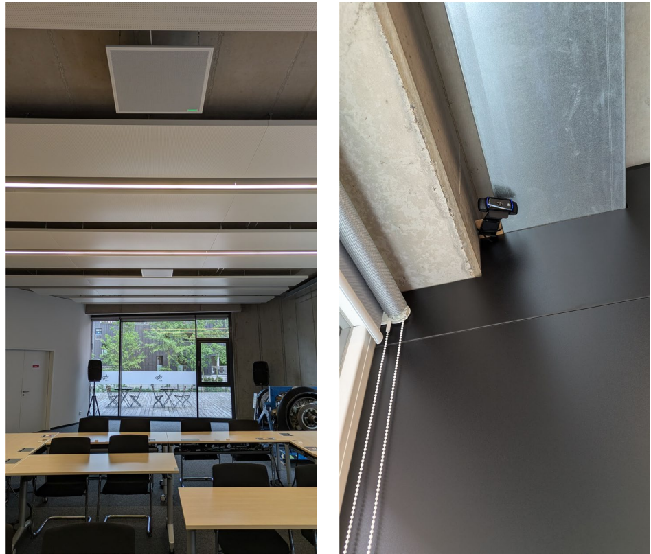
(a) Ceiling microphones in the center of the room. (b) Webcam behind the speaker's table facing towards the plenum.
