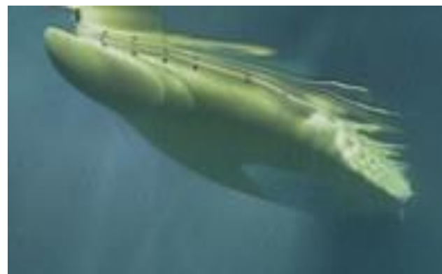
Figure 12: Snapshot of air layer on LNGC (17.5 knots)
