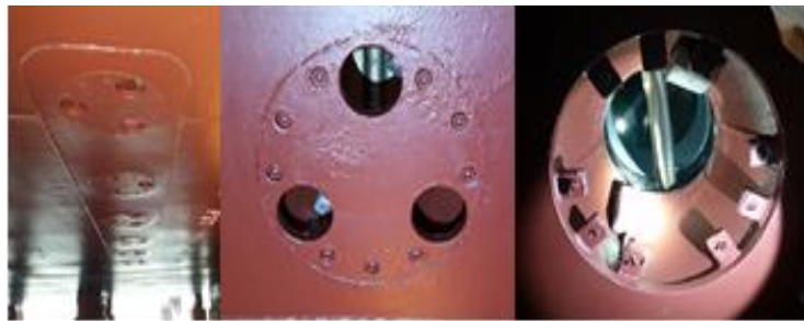
Figure 15: Air injectors on the hull bottom
