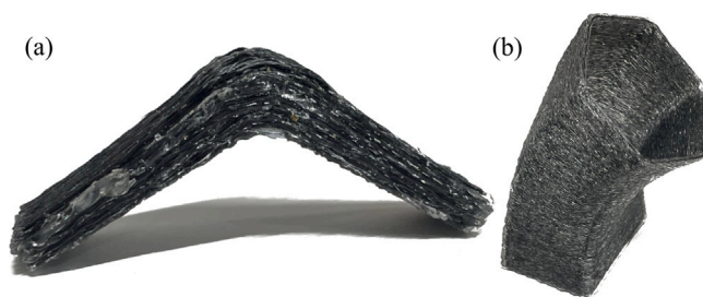
Fig. 10. Results for printed tests parts to evaluate applicability of the process with layer height variation. (a) V-Bracket with dimensions 10 mm x 43.5 mm x 17.3 mm and (b) Tube structure to demonstrate the variation of layer thickness and reduction of necessary layers and non-planar deposition with dimensions 42 mm x 52.5 mm x 76.7 mm.
