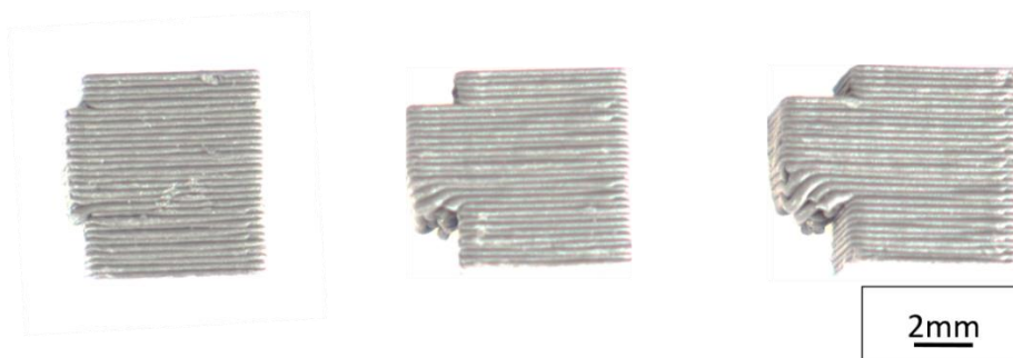
Figure 2: Representation of the 0.5 mm (left), 1.0 mm (middle) and 2.0 mm (right) overhang and defects
