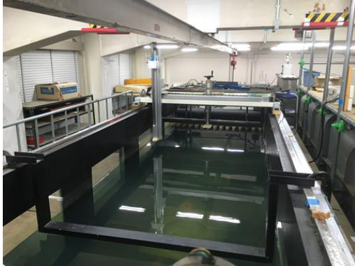
Figure 4: Circulating water tank
