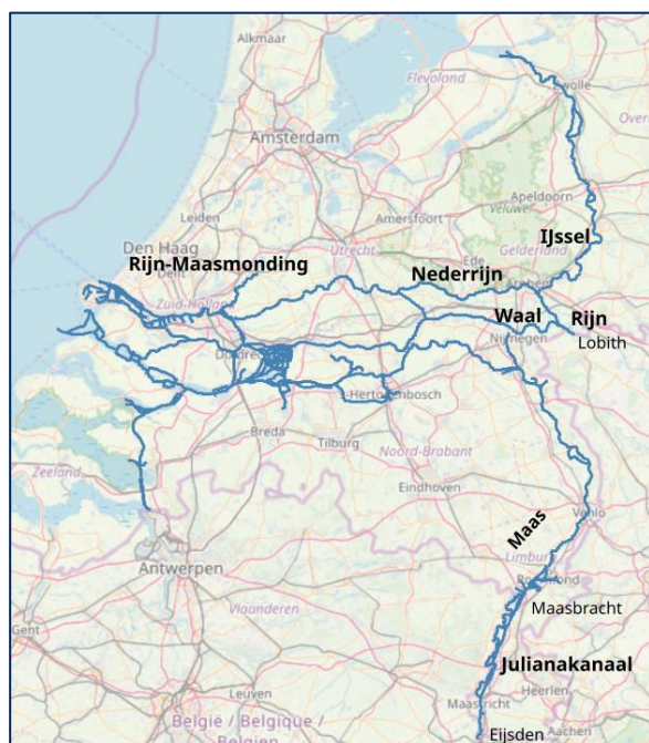
Figure 2: River branches in the combined 1D SOBEK model of the Maas/Meuse, Rijn/Rhine and Rijn-Maasmondig/Rhine-Meuse-delta. Several other locations that are mentioned later in this paper are also included.
