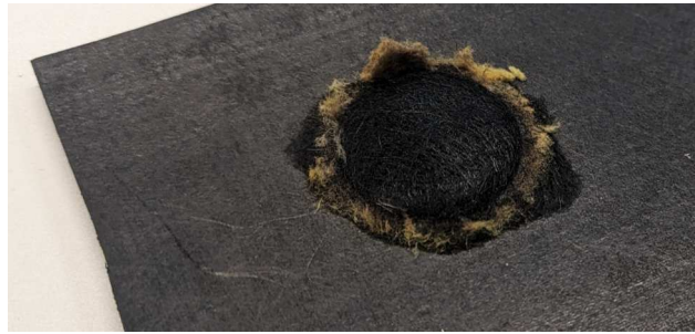
Figure 2: Expanded sample (yellow material detached from the insulation)
