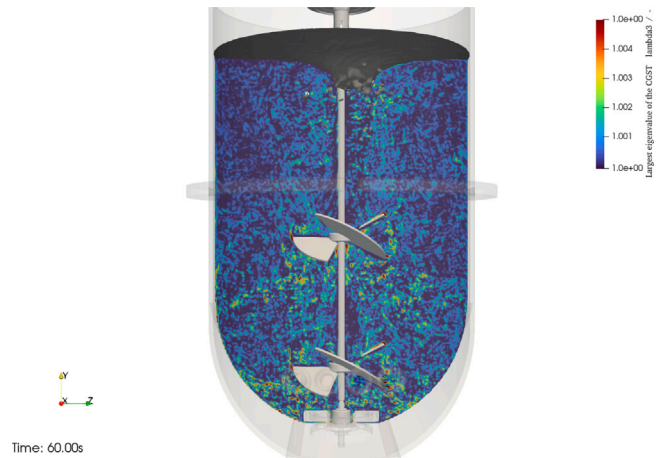
Fig. 9. Contour of the largest eigenvalue \lambda_3 of the CGST for the case n = 150 \text{ rpm} on the x -plane.
