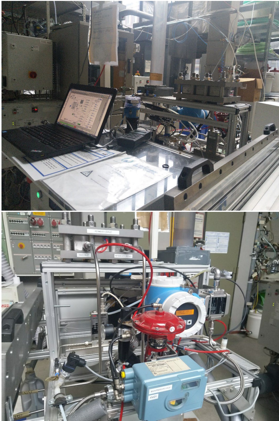
Figure I-1: Sterlitech membrane cell setup used for crossflow filtration experiments at Institute for Water Resources and Water Supply, TUHH
