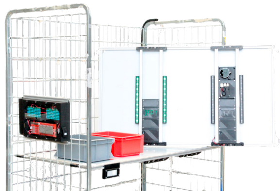
Fig. 6. Retrofitted Delivery unit with a presented smart sensor board. The smart board is equipped with different sensor modules such as camera and BLE modules. Additionally, the slide-in trails are equipped with pick-by light modules that indicate to be loaded/unloaded areas. On the side of the delivery unit, the battery package is mounted.
