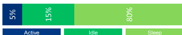
Fig. 5. Distribution of power modes from the smart delivery units sensor modules and CPUs. Based on a 10h transportation procedure.
