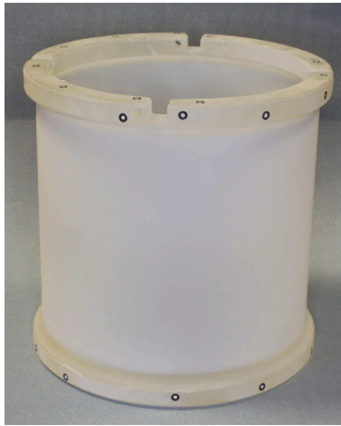
Fig. 7. One of the polymer cylinders from [8], of which the imperfections are used to generate random samples.
