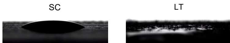
Figure 5.25: Wetting behaviour of diiodomethane for the solvent cleaned (SC) and laser-treated (LT) configuration.
