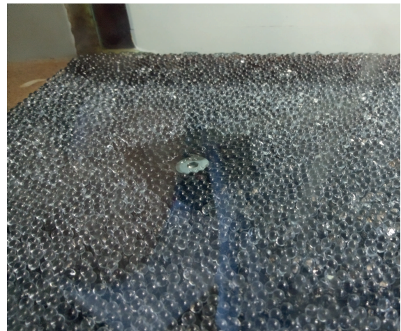
(b) Fixation by screws of PVC-plate with glued particle layer
