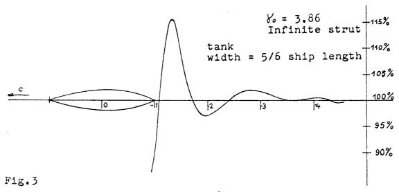
Ratio of Calculated Resistance  $R_t^{(2)}(x)$  from Transverse Cut Analysis [6] (Wave Elevation and X-slope) to Asymptotic Value  $R^{(2)}$
