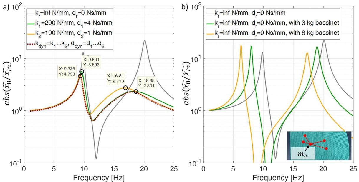
Figure 5. Amplification function at Point P8 a) for stationary adjustable interfaces and dynamical adaptive interfaces and b) for different product variants.
