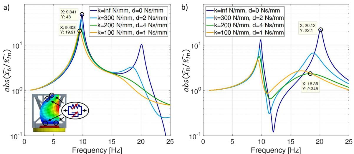
Figure 3. Amplification function of the simulation model with different interface stiffness and damping at Point 6 and 8.
