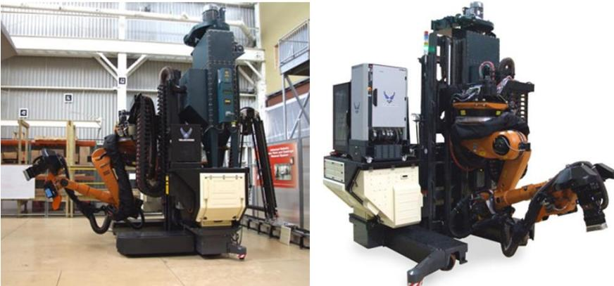
Abbildung 25: LCR-Systems "Laser Coating Removal for Aircraft" [LCRI4]
