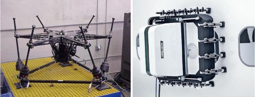
Abbildung 23: links: PushCorp "Scarfing Tool for Automated Repair" STARC [ErGo95], rechts: DMG Mori „MobileBlock“ [Feu15]
