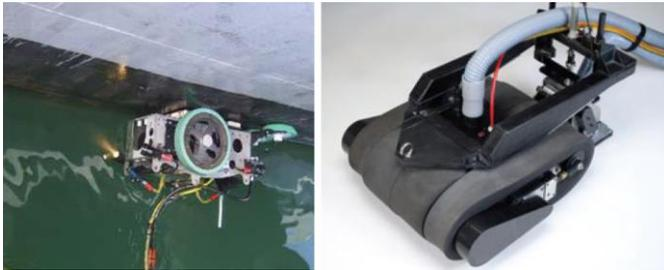
Abbildung 21: links: Magnetic Hull Crawler (MHC) [Cyb11], rechts: The Climber [Gil10]
