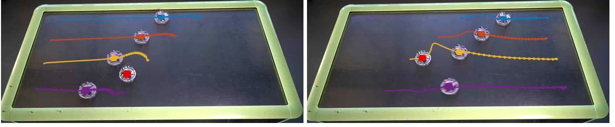
Figure 5.11: Camera images of a point-to-point transition with a dynamic obstacle and embedded DMPC. Solid lines with dotted markers are predicted trajectories and lines without markers show the latest closed-loop trajectories. Pictures by Roland Schwan.
