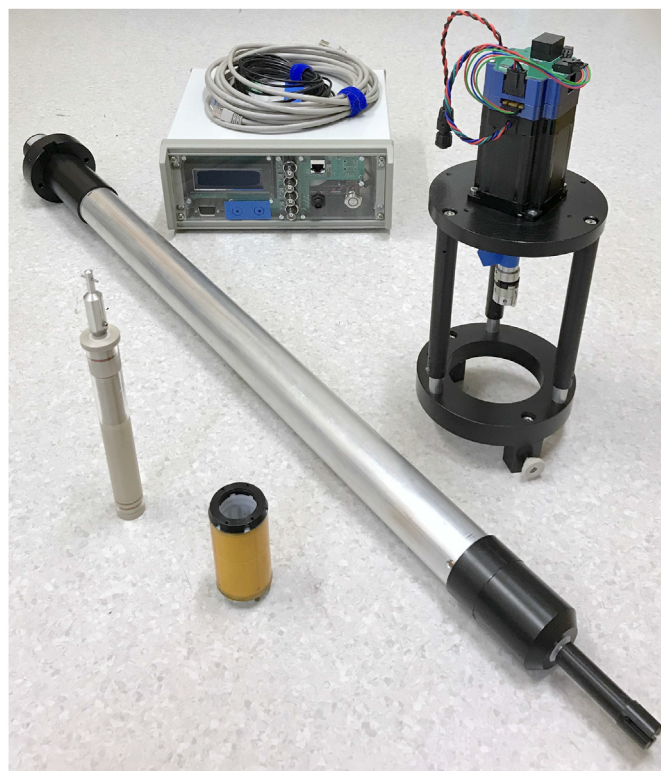
Fig. 3. Components of Magritek Rheo-NMR kit such as controller module (top center), motor, gearbox, and mounting unit (top right), drive-shaft (diagonal), shear device (left), and RF coil (lower left). Reproduced with permission from Stevenson (2018).
