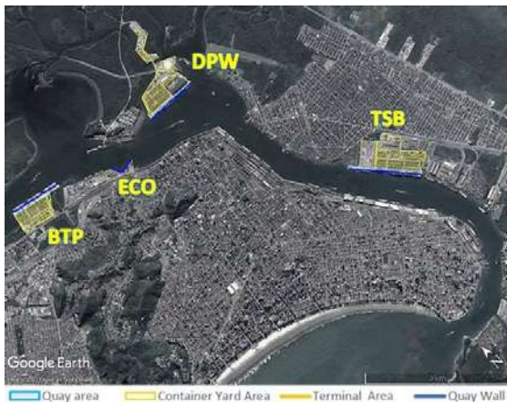
Figure 2: Aerial view of the Estuary of the Port of Santos, highlighting the access channel and major logistics infrastructure of the container terminals, such as Brasil Terminal Portuário (BTP), DP World Santos (DPW), Tecon Santos Brasil (TSB), and Ecoporto (ECO). Source: Google Earth (July 2022).
