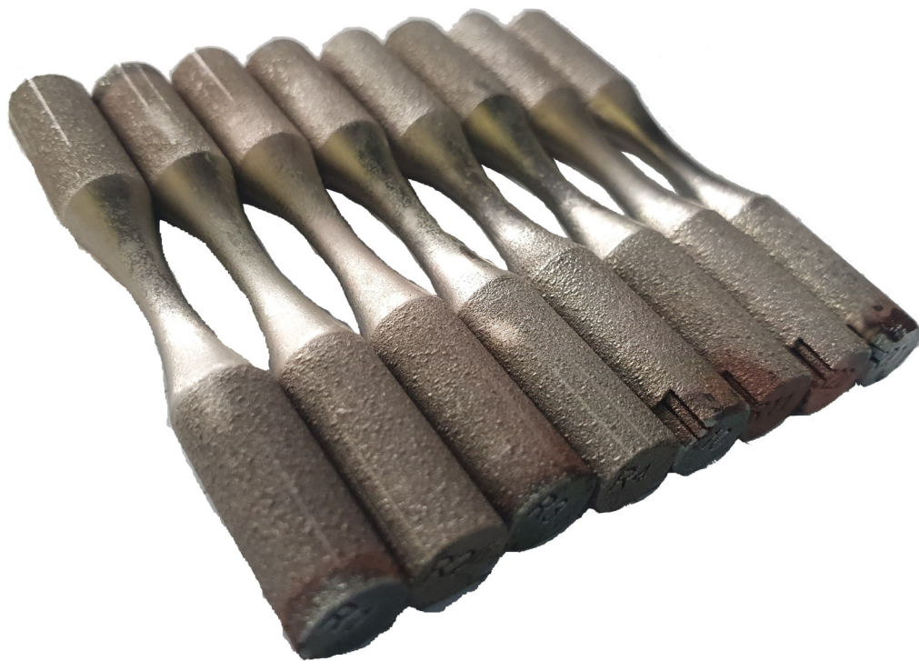
Figure 5.19: Additive manufactured samples provided by the TUM and coated with Cu/Ni NMM
