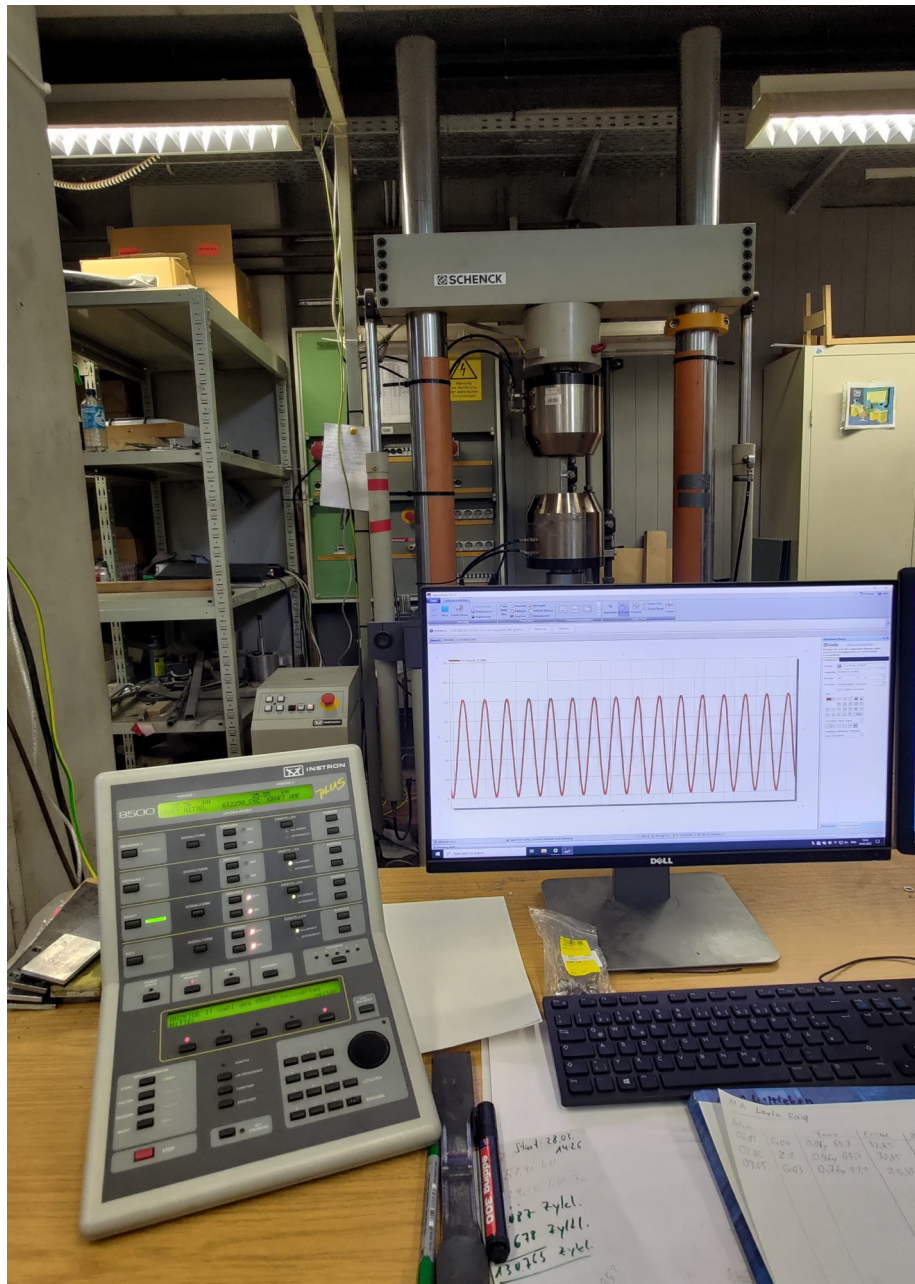
Figure 3.4: Servo-hydraulic test machine
