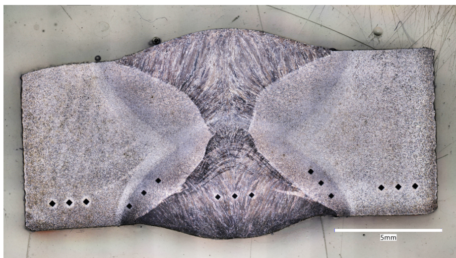
Figure 3.3: Etched micrograph of the weld
