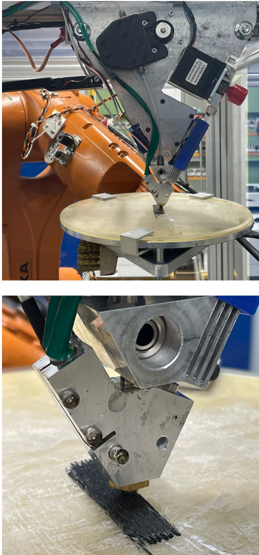
Fig. 9: Physical realization of the printhead during functional verification; part cooling vent and fan flipped up for better visibility. Printed part shows cuts
