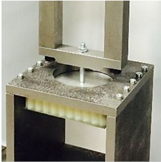
Figure 7. Basic test setup of a pull-out test.
