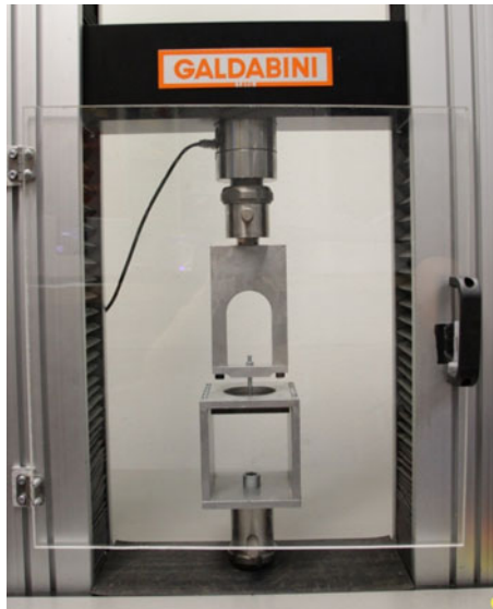
Figure 12. Test setup of the pull-out test.
