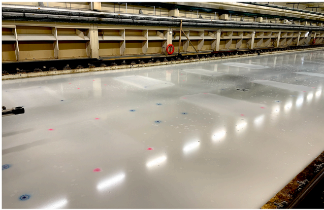
Fig. 15. Oblique view of the small measurement areas on ice sheet No. III after surface modification. The extent of the areas was marked on the ice with colored chalk spray. A change in surface appearance from glossy (intact surface layer: surroundings and quadratic reference areas) to matte (thermohaline-melted surface layer: elongated areas) is evident.
