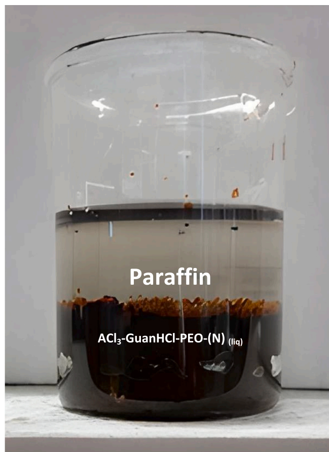
Fig. 1. A typical \text{AlCl}_3 guanidine HCl DES.
